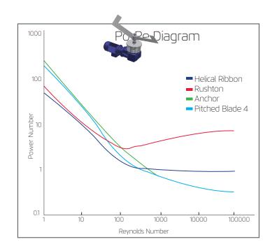
D – Impeller Diameter [meter] N – Revolution per Second [1/sec] r – Density [kg/m³]
